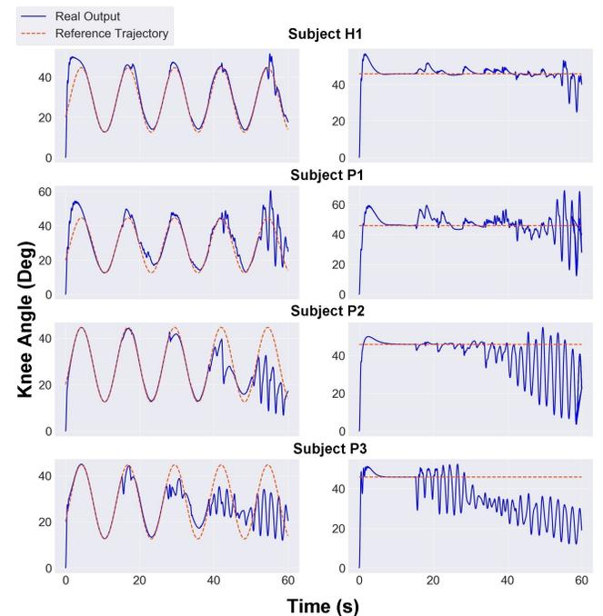
Fig. 5: Analysis of system responses using IGA tuning considering critical non-idealities.
