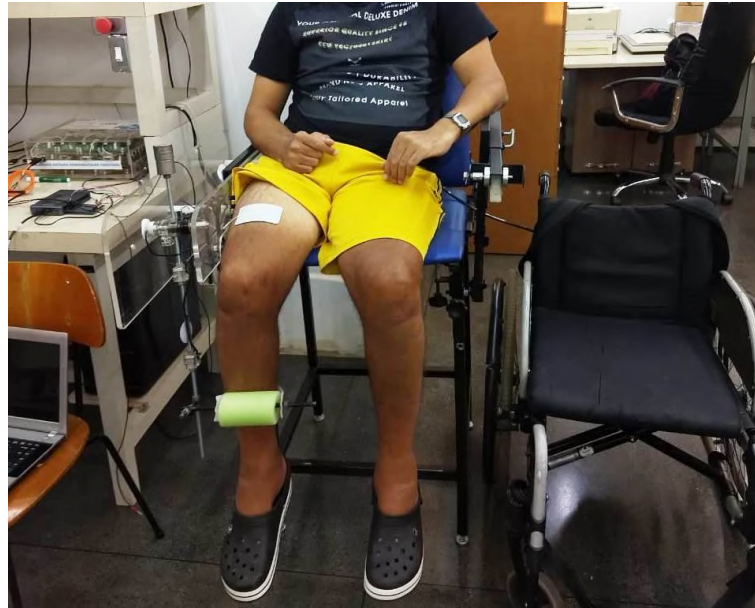
Figure 20 - Individual P2 in the instrumented chair.
